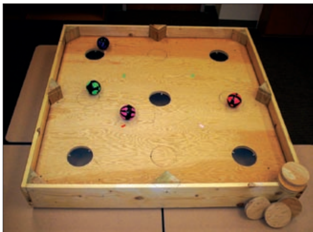
Fig. 1. Photograph of the experimental setup. The Squiggle Balls roll about until they are “captured” by falling into one of the uncovered holes.
